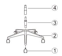
Press Casters (1) into holes of the Base (2). Insert Seat Post (3) and Seat Post Cover (4) into the center hole of the Base (2).
