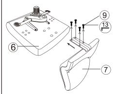
Attach Backrest (7) to the Seat (6) using 4pcs Screws and 4pcs Washers (9). Tighten securely with enclosed Allen Wrench (13).
