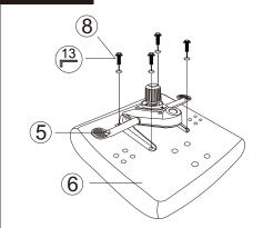
For easy assembly, place Seat (6) face down on a flat surface. Attach Mechanism (5) to Seat (6) using 4pcs Screws and 4pcs Washers (8). Tighten securely with enclosed Allen Wrench (13).
