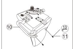
Insert 2pcs Screws (11) into the rear holes of Armrest (10) as shown, attaching Armrest (10) to Backrest first. Do not fully tighten these 2 screws until told to in Step 5.
