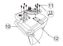
Attach Armrest (10) to Seat using 8pcs Screws (11) as shown. Tighten securely with enclosed Allen Wrench (13). Now fully tighten the 2 screws (11) from Step 4 into the Backrest. Attach 2pcs Arm Screw Caps (12) to cover exposed holes on Armrest (10).
